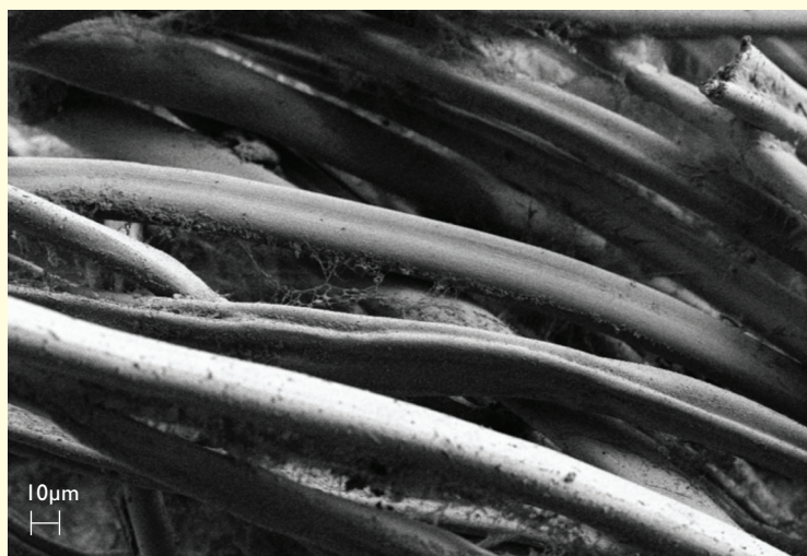
Fig 2. Drawtex hydrated under SEM at 1000x magnification
